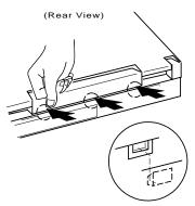
**Note:** When replacing the indicator, insert the flexible cable straight into the connector until the head of the cable stops. Slide both ends of the latches at the same time to make sure that the cable is correctly inserted.
